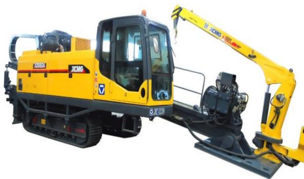
Horizontal Derectional Drill
